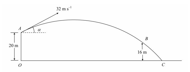
A particle *P* is projected from a point *A* with speed 32 m s<sup>-1</sup> at an angle of elevation  $\alpha$ , where  $\sin \alpha = \frac{3}{5}$ . The point *O* is on horizontal ground, with *O* vertically below *A* and *OA* = 20 m. The particle *P* moves freely under gravity and passes through a point *B*, which is 16 m above ground, before reaching the ground at the point *C*, as shown in Figure 4.
