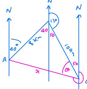
2 = 8 + 10 - 2x 8x 10 cos 90  $x^{2} = 164$ x = 1164 = 12.8 Km Sine rule  $\frac{x}{Sin90} = \frac{8}{Sin0}$  $\frac{\sin 40}{12.8} = \frac{\sin 2}{8}$ Singo 8 = Sind S = Sinta 0 = Sin" ( ) Q = 39° (n'est degree) Bearing = 360 - (39+50) = 271°
