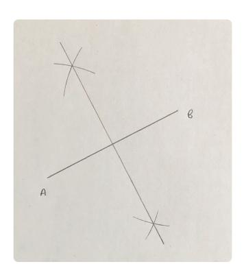
Construct a perpendicular bisector of a line AB
