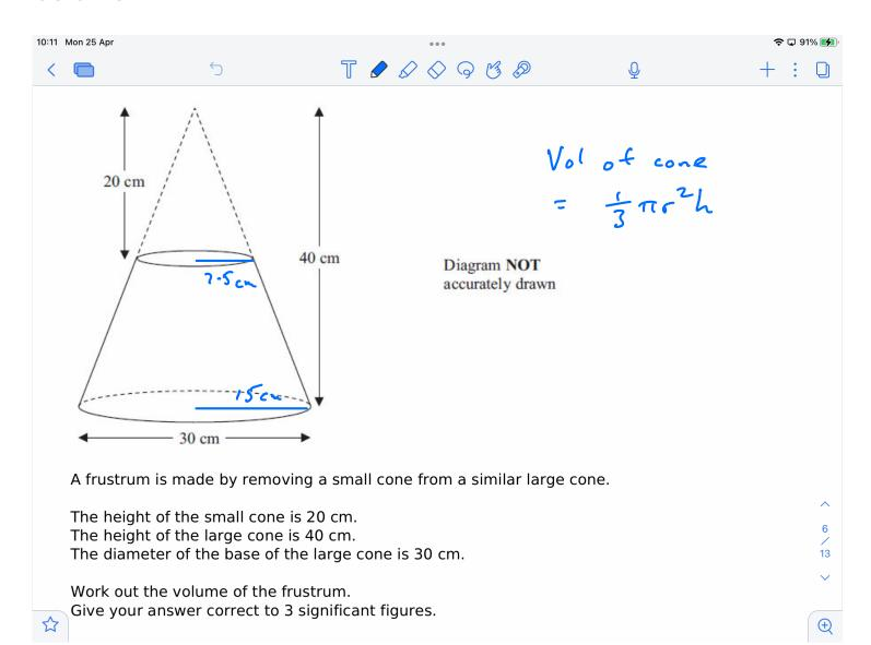
Vol of Frustum = Vol of large cone - Vol of small cone
